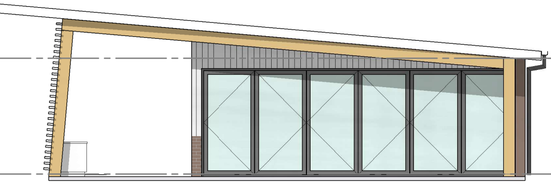
3 SPORTS PAVILION - REAR ELEVATION SCALE 1 : 100
